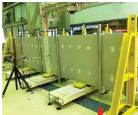
Test quasi-statico out-of-plane
