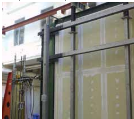
Test quasi-statico in-plane
